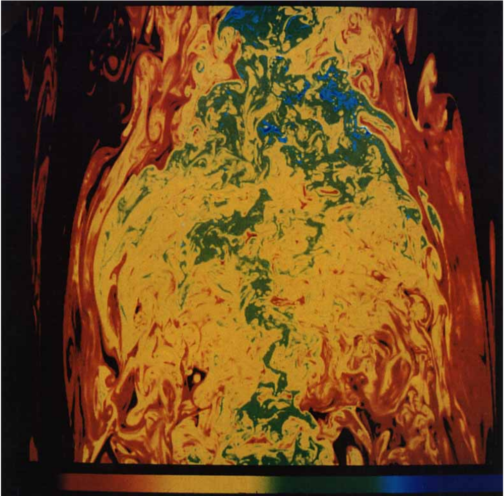
FIGURE 8. Details of time evolution of the instantaneous radial concentration profile within a large structure in a jet at Re=9600 , x/d=150 . Total time 10.67 s.
